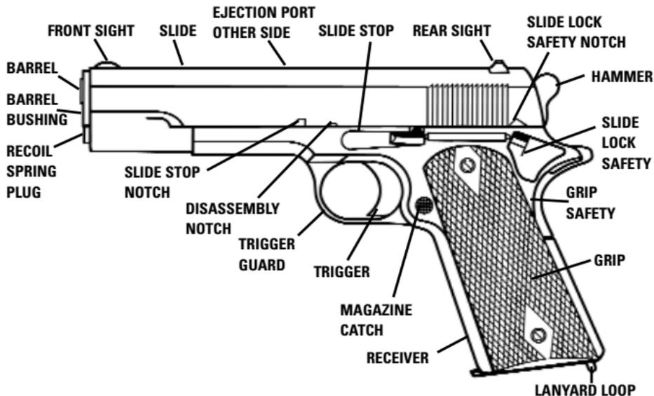
**FIGURE 1 - USFA AUTOMATIC PISTOL**
