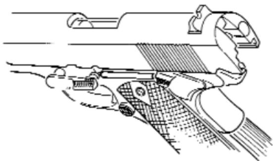
**FIGURE 10 - INSTALLING SLIDE STOP**
