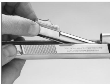
Lift out the barrel.
