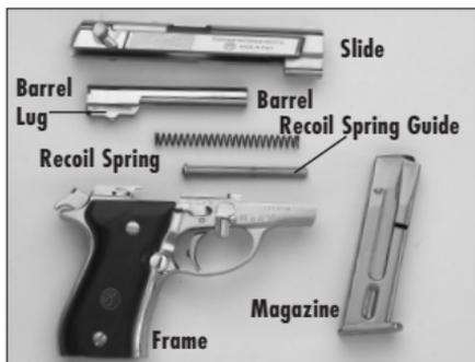
Disassembly to this point is sufficient for normal maintenance of your pistol.
