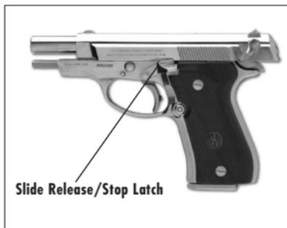
Depress the slide release/stop latch.
